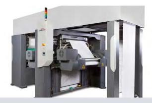
The reel change and web transfer to the new core is then automatic. As for all models, operational data is shown on the HMI of the rewinder and motorized reel sidelay is included as standard. Additional options are as for the CR-W.
