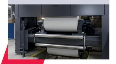
Rather than using a pivot frame to correct the position of the web, the Contiweb FD web guide function is integrated into the sidelay movement of the split reel carrier arms, so that the position of the reel as a whole is corrected. Thus non-uniformities in web tension are avoided. An additional advantage is that the web guiding is performed before the integrated infeed at the low tension side of the paster.
