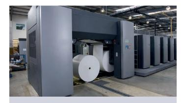
The Web Data system weighs each paper reel with its wrapping and again with the wrapping and waste paper removed. Additional information like reel diameter, paper grade, form and shift identity, and start and stop times can be entered by operators or acquired automatically from the splicer or paster controls. The result is a comprehensive collection of data that can be used to calculate detailed reports on waste, production efficiency and faults related to paper and splicing.
