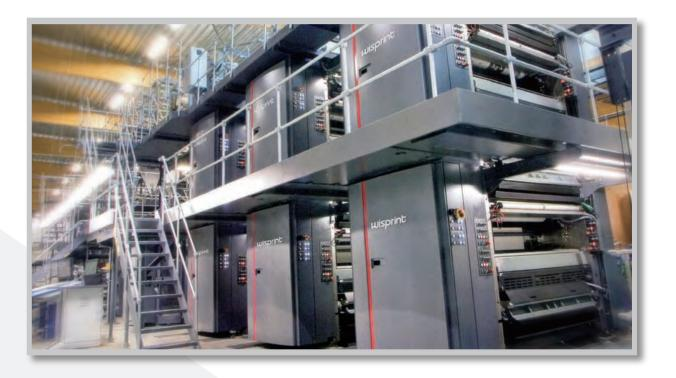
The Wisprint 80 press is recognized worldwide for high-level print quality and productivity. It offers the flexibility of a single-width press while the two-plate-around configuration allows maximum productivity with printing speed up to 80,000 copies per hour.
