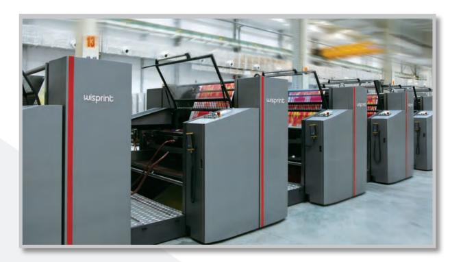
Our Aqua Stream is designed to meet the growing demand of environmental friendly packaging. Capable of printing on paper or board, the Aqua Stream uses water-based flexographic printing process. This press is modular in design and can be easily configured to meet customers' printing needs. Optional turner bars allow for reversing side printing if required. In additional to printing packaging, customers are also using the Aqua Stream to produce environmental friendly books.
