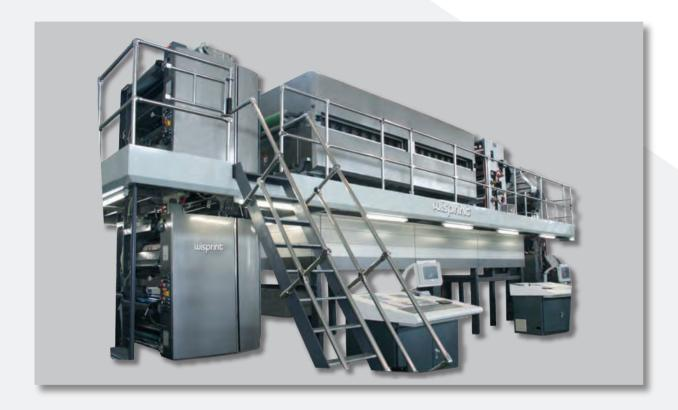
The MV400 is designed as a cost effective semi-commercial press. The press is designed as a 4Hi configuration and combined with a dryer as a compact semi-commercial press. The press can print on paper, coated or LWC paper and can produce value added high-quality output.
