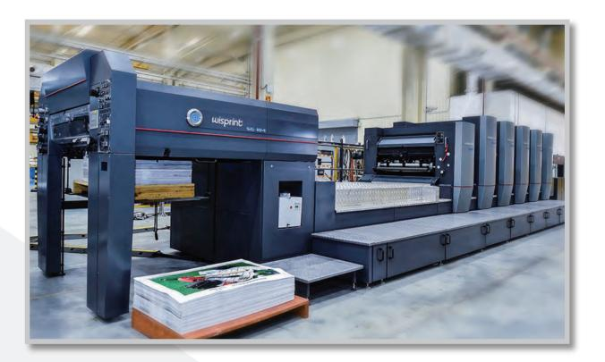
Our proven SG-104 Sheet Fed Press is now available with additional print technologies in order to enhance the value of the printed products. These improvements include a varnish print unit and cold foil print unit. The additional print technologies greatly enhance the appearance, quality and value of the printed products.
